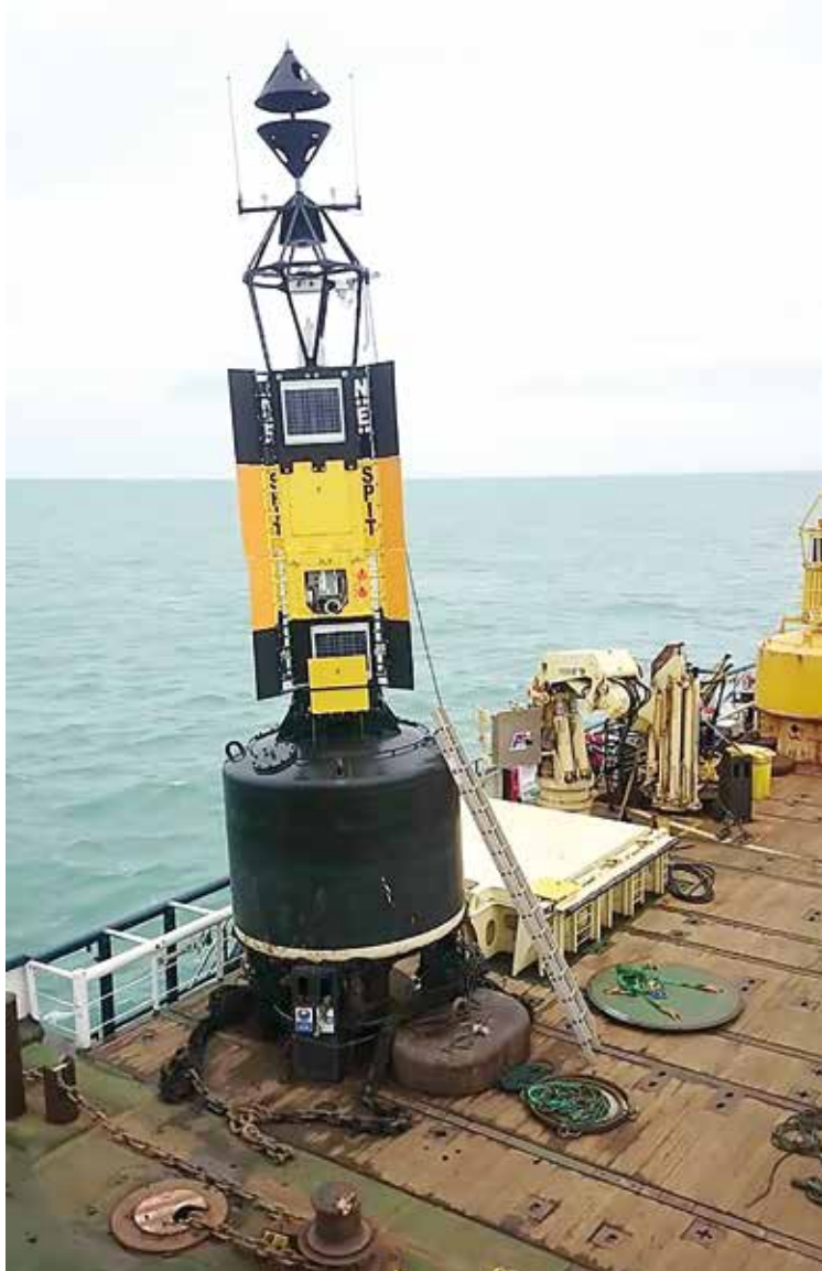
Above: NE Spit buoy on board THV Galatea for installation of Met-Hydro equipment
