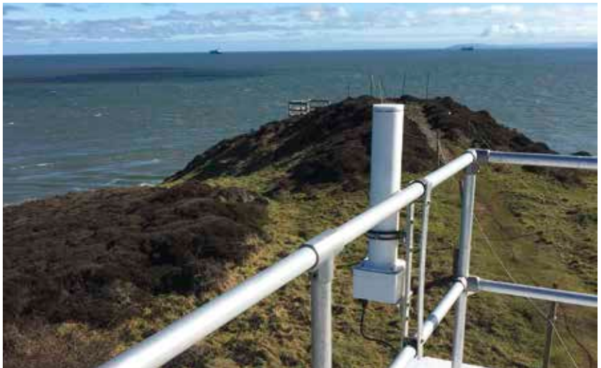
RIMNET's coastal monitors are designed to detect the threat of radiation from an overseas incident
