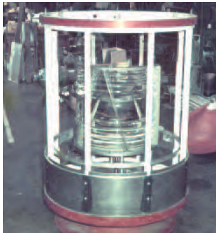
Above: Creation of new equipment in an effort to provide cost-effective and reliable aids to navigation would not have been possible without input from the Drawing Office and Blackwall Workshops. This example shows a lantern being assembled at Blackwall for Northfleet, one of the Thames river lights.
