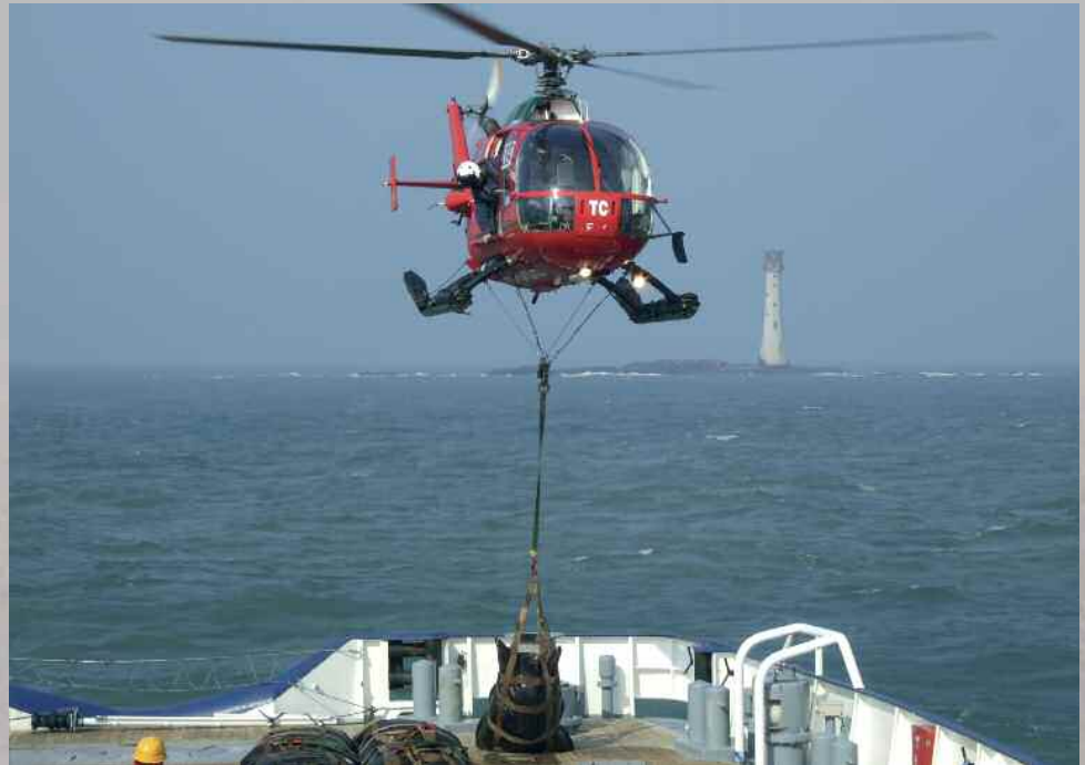
Above: The Trinity House helicopter working with a district tender prepares to deliver oil in a pillow tank to Smalls. Photo: Mike Yaxley.
